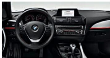
The sport leather steering wheel with red stitching and the speedometer and rev counter design featuring red chronoscales are exclusive to the Sport Line.
