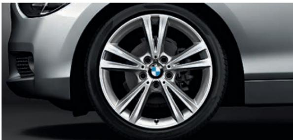
The new BMW 1 Series comes standard with 16" steel wheels with wheel covers, 6.5 J x 16 with 195/55 R 16 tyres. The BMW 120d is available with 7 J x 16 alloy wheels with 205/55 R 16 tyres (pictured here with 18" light alloy wheels Double-spoke 385 with mixed tyres).
