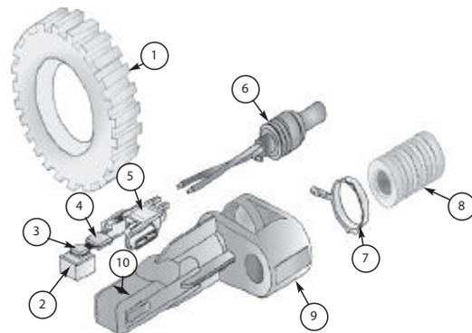
As the high portion of the pulse wheel approaches the sensing element a deflection of the magnetic field stream is created. This creates a resistance change in the thin film ferromagnetic layer of the sensor element.
