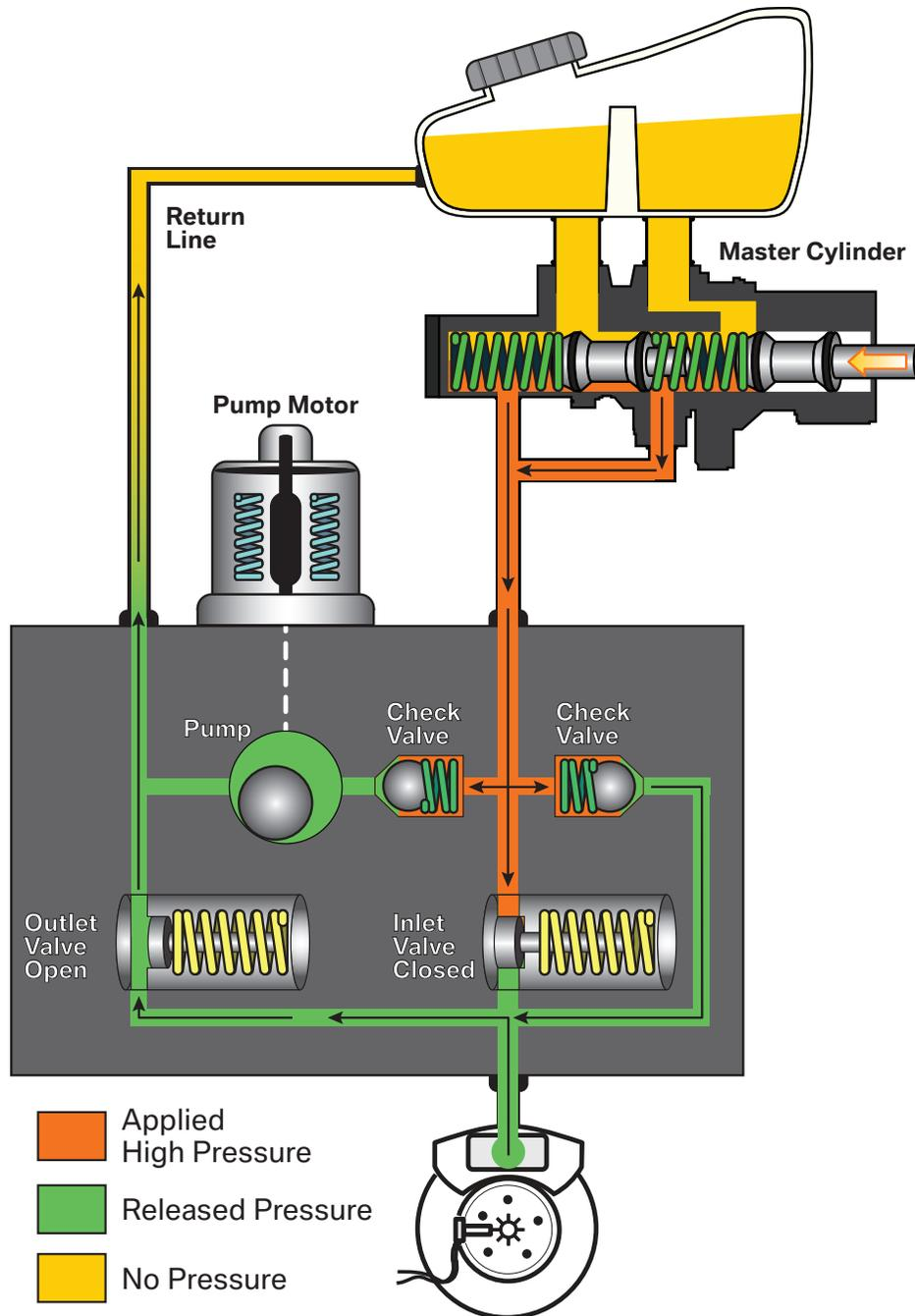
**Typical ABS/DSC Hydraulic Schematic**
