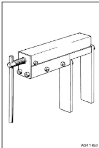
**Brake line bending tool (34 5 100)**
