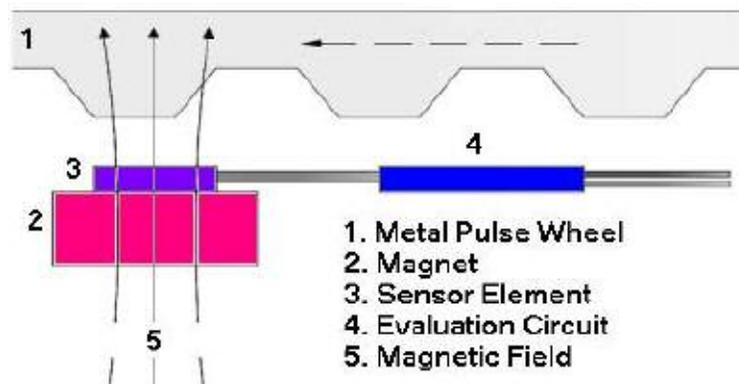
The sensor element converts the changes in resistance into voltages.
