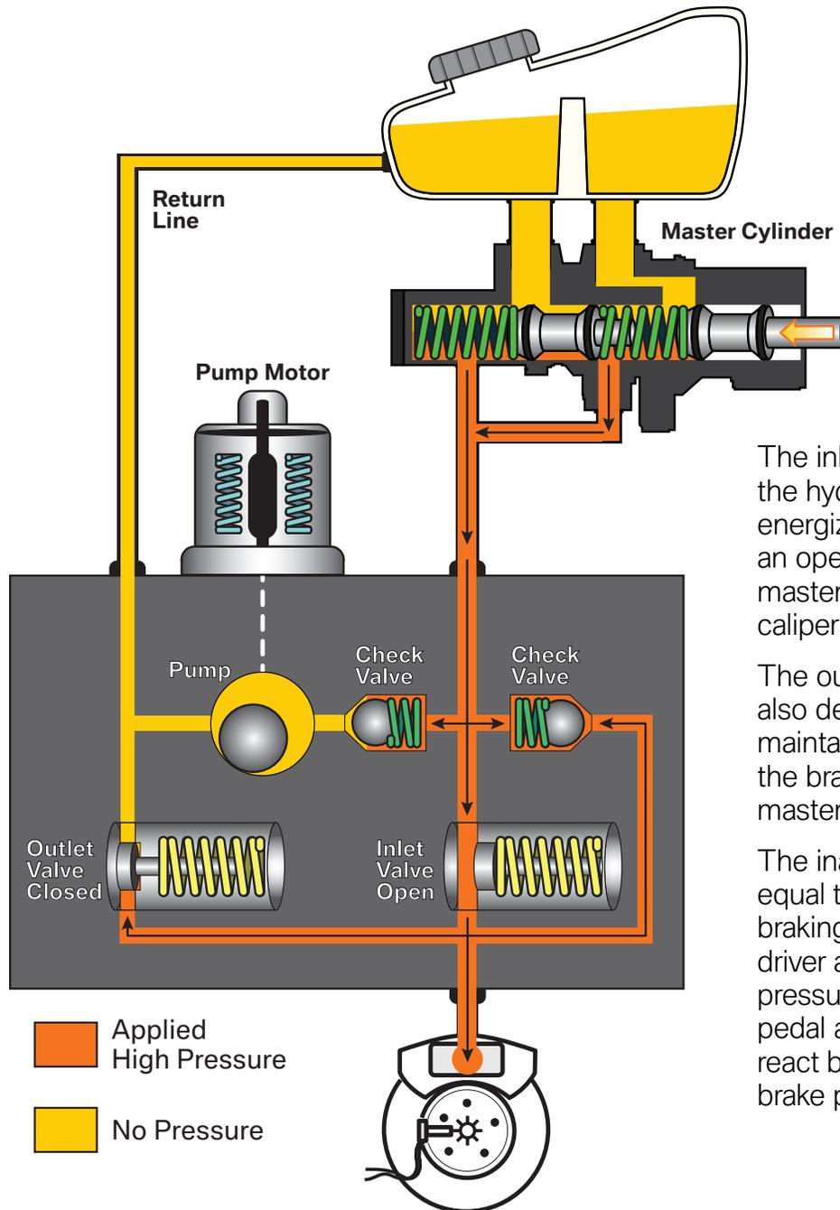
The inlet solenoid valves of the hydraulic unit are de-energized. This maintains an open passage from the master cylinder to the brake calipers.
