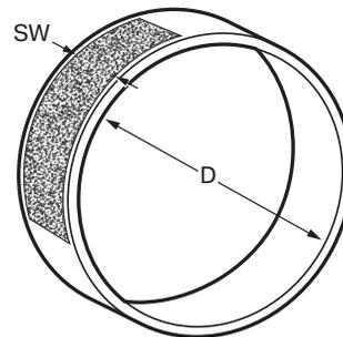
Most passenger cars use a swept area of about 200 square inches of lining for every 2,000 lbs of vehicle weight. Road racing vehicles that place a severe load on their brakes will use double the swept area or about 400 square inches of lining for every 2,000 lbs of vehicle weight.
