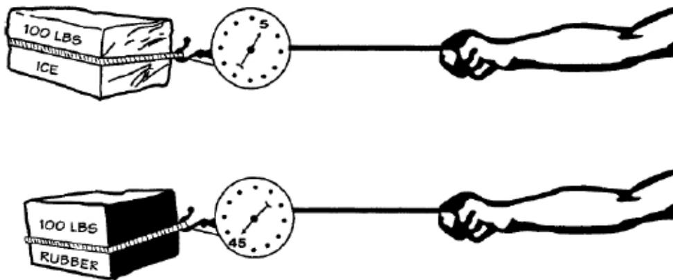
The above example illustrates how the type of friction surface and the material can influence the coefficient of friction (COF).
