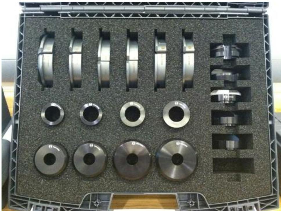
Rear Wheel Bearing Race-Removing Kit 83 30 0 493 416
