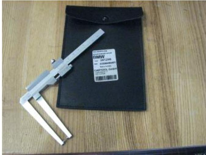
**Handbrake shoe release tool 83 30 0 492 488 (34 4 000)**
