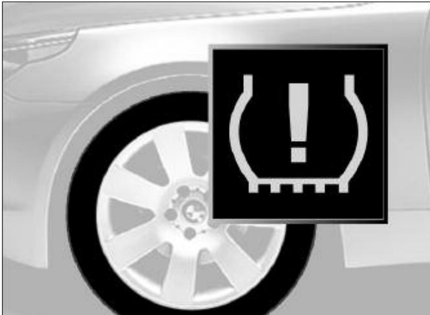
The main function of the system is to monitor the tire pressure during vehicle operation. The most important auxiliary function of the system is the option of independently detecting the wheels (vehicle's wheels) mounted on the vehicle and their position.
