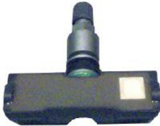
Electronic assignment of the wheel electronic modules is not carried out until movement is detected. This is to avoid any signals from vehicles in close proximity. Especially vehicles which are equipped with similar TPM systems.
