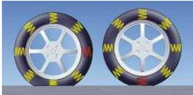
Also, checking the radial runout of the tire (when unloaded) does not give an indication of radial force fluctuations. The only method to accurately check for radial force variations is to use the GSP97BMW wheel balancer.
