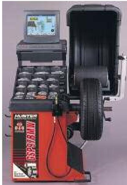
Lateral as well as radial force fluctuations occur. These can be traced through the sideways wobble of the wheel. Lateral means sideways. Lateral force fluctuations have less of an effect on harmonics than radial force fluctuations.
